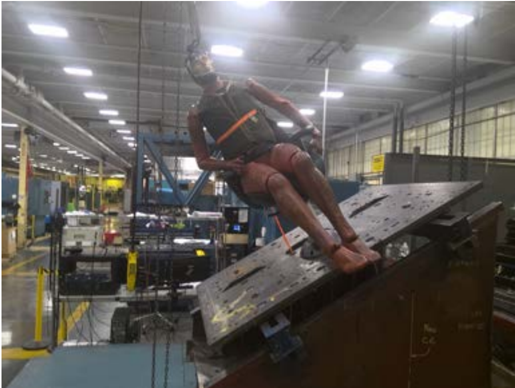
Photo 11 - File No. T20230905-5547 Pretest, 30 degree Side Down, setup
