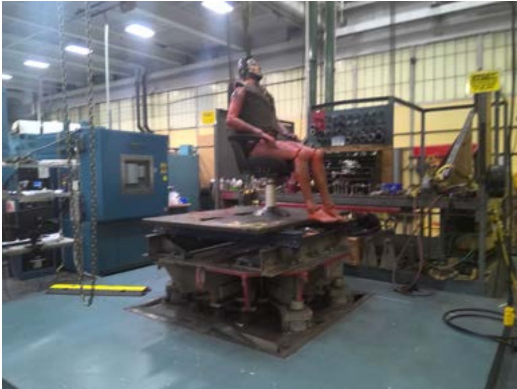
Photo 5 - File No. T20230905-5539 Pretest, test item and dummy setup in vertical orientation
