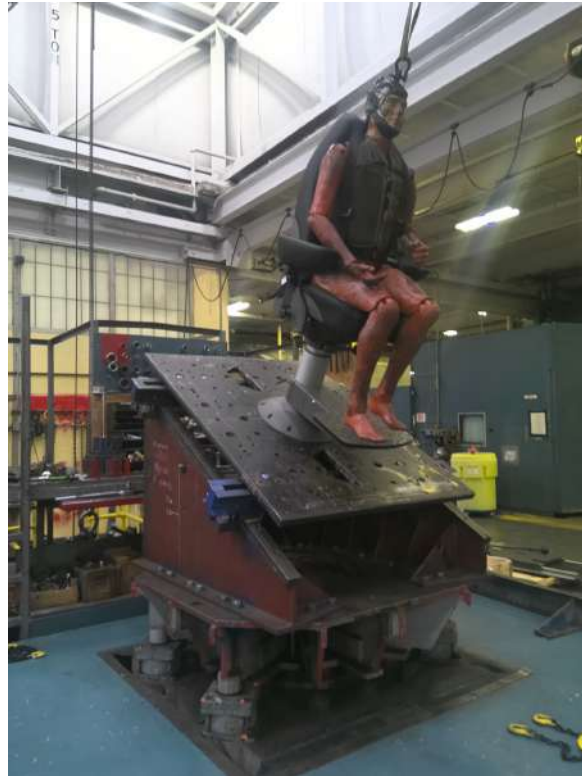
Photo 9 - File No. T20230929-6159 Pretest, 30 Degree Front Down Setup
