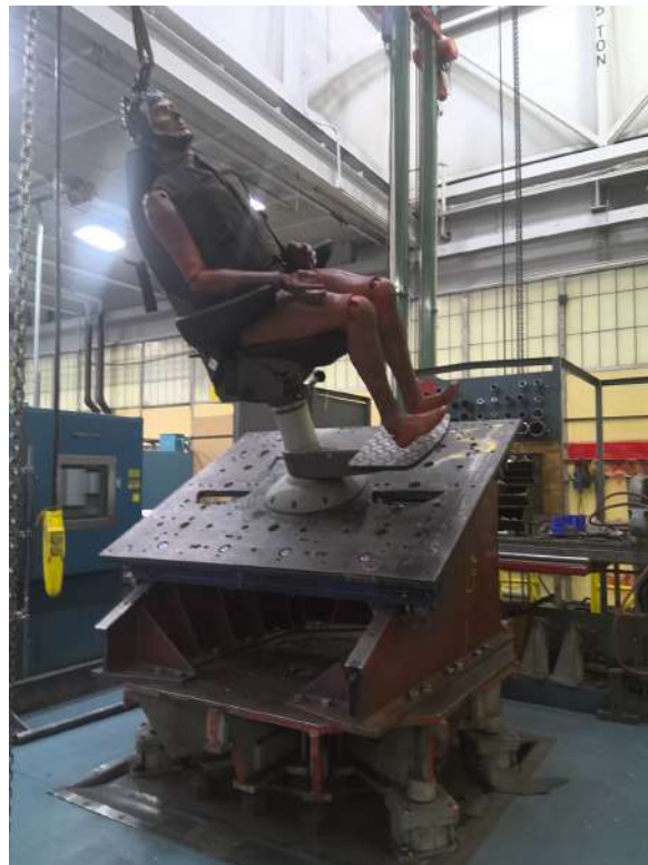
Photo 12 - File No. T20230929-6171 Pretest, 30 Degree Side Down Setup
