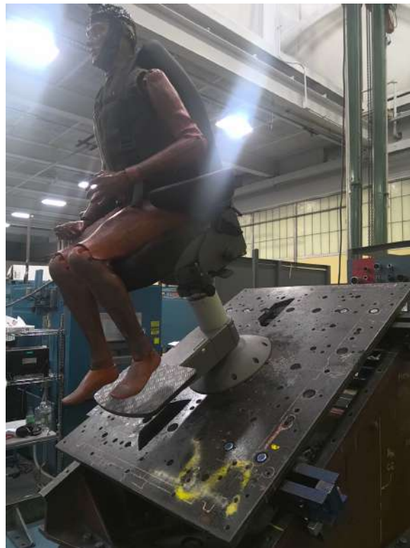
Photo 10 - File No. T20230929-6160 Pretest, 30 Degree Front Down Setup
